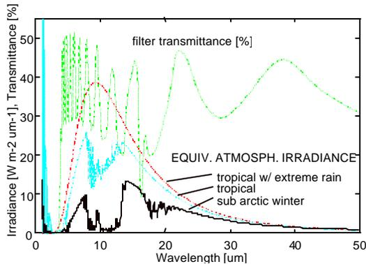
**Typical Atmospheric IR spectrum**
