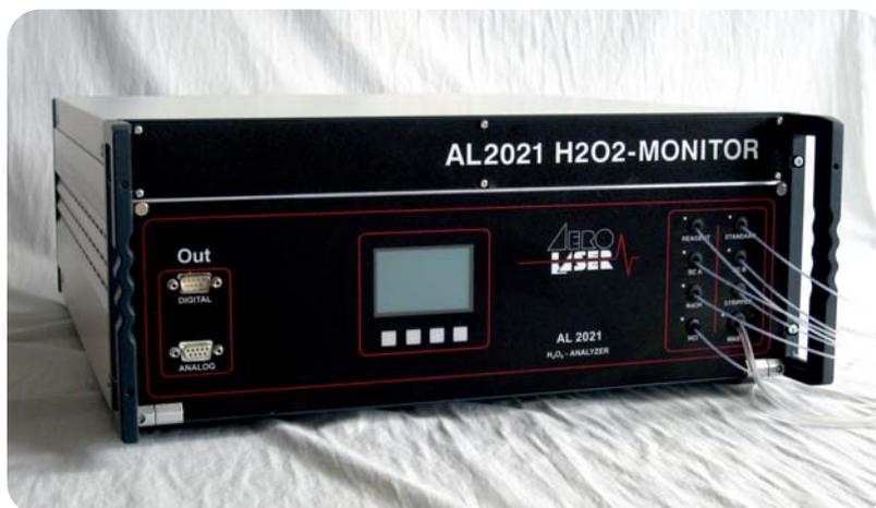
The H<sub>2</sub>O<sub>2</sub> monitor AL2021 from Aero-Laser has an extraordinary high sensitivity and a unique low detection limit of 100ppt (parts per trillion) for gaseous samples and 100 ng/liter (eq.  $2 \times 10^{-9}$  molar) for liquid samples, respectively. The complete chemical processing, including gas stripping, is integrated into the instrument.
